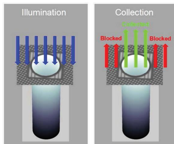
In order to further increase the variety of independent channels, we implement measurement schemes based on the notion of dark-field (DF) detection. In DF measurements, the optical system is designed so that light going through 'simple' reflection from the sample is blocked before detection. The meaning of 'simple' here depends on the specific type of obstruction used on the light return path, which can have several common variations:
