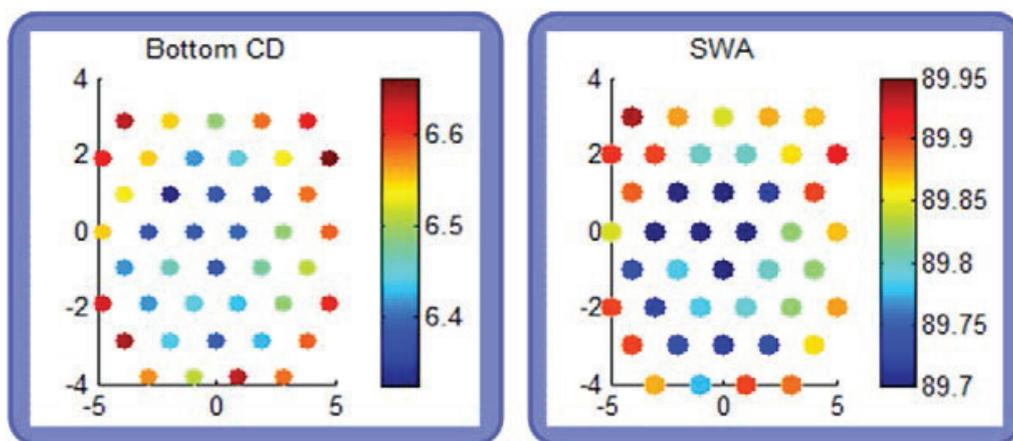
TSV profile characterization using dark-field reflectometry.
